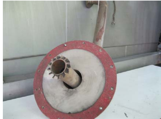
Figure 3. Detail of the burner construction, pointing out the axial blades for the swirling of the tertiary air.
