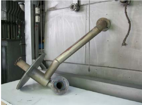
Figure 1. General view of the pulverized state sawdust burner
